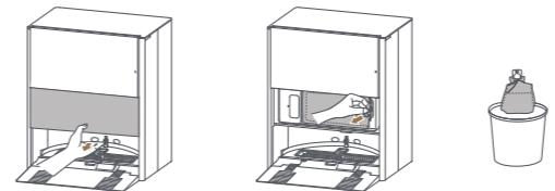
**Note:** Pulling upwards on the handle will seal the bag to prevent the dust and debris from accidentally falling out.
