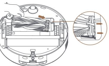
4. Align the front end of the brush guard with the slot, insert it downwards in an inclined way, and then press it into place.
