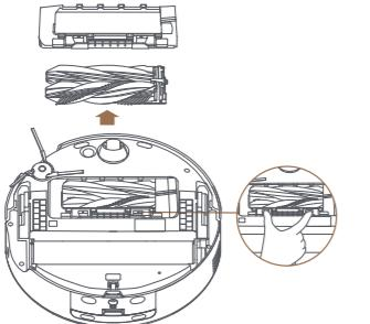
2. Pull out the brushes as shown in the figure. Use a proper tool to remove any hair tangled in the brushes. After cleaning, push the brushes firmly into the main brush holder until they click into place.
