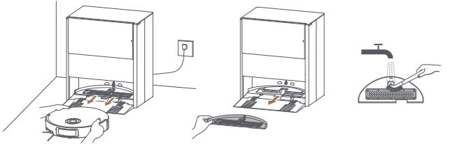
**Note:** The heating module under the washboard may retain residual heat. To prevent scalding, be careful when removing the washboard.
