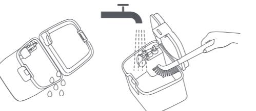
**Note:** The float ball in the used water tank is a movable part. Do not apply too much force when cleaning it to avoid damaging it.
